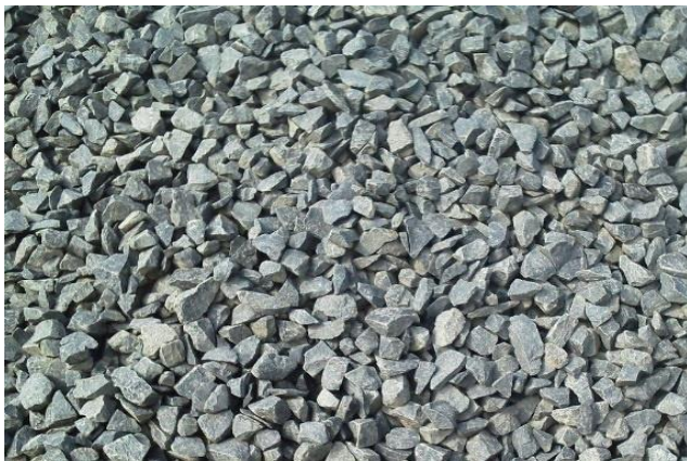
Uniformly sized, highly angular crushed stone
