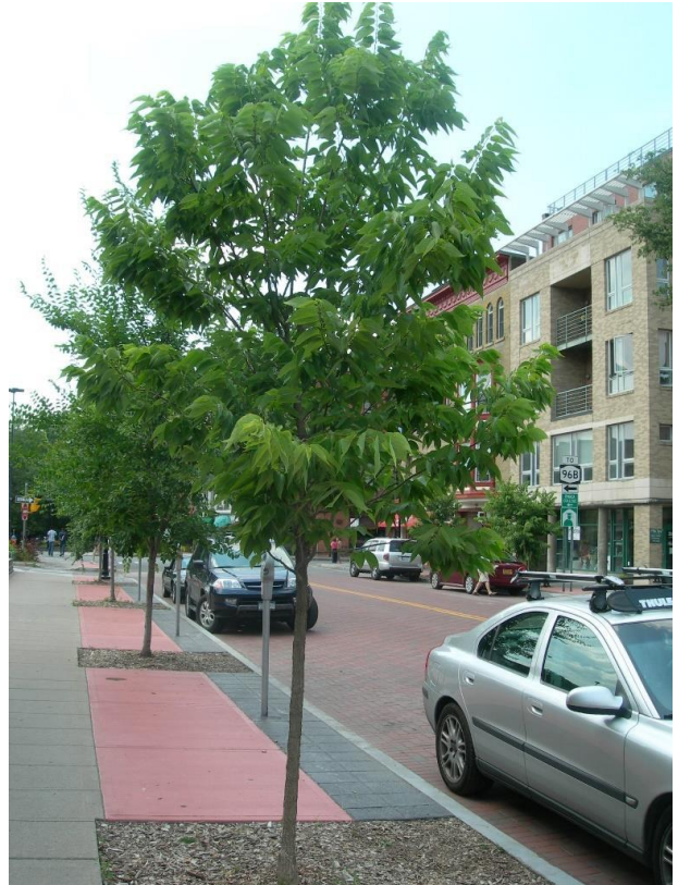
In urban situations where tree lawns are not practical, pavement over CU-Structural Soil® allows street trees to share a large-volume, continuous strip of useable soil, as seen here in Ithaca, NY.
