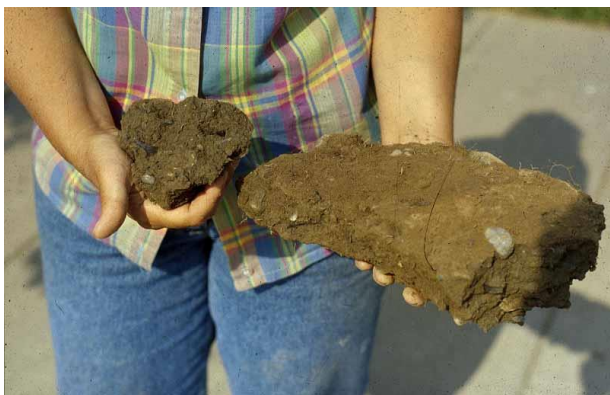
Severely compacted soil that is "dense as bricks" and not conducive to tree root growth
