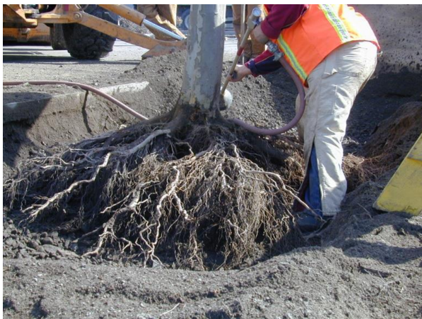
Excavation of a tree growing in CU-Structural Soil®
