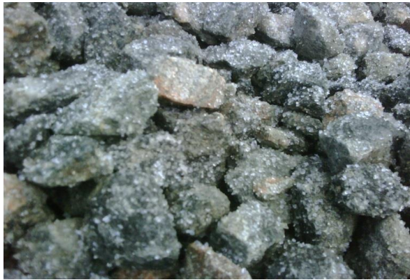
Close-up of angular stone with Gelscape® Tackifier applied (prior to admixing with clay loam soil)
