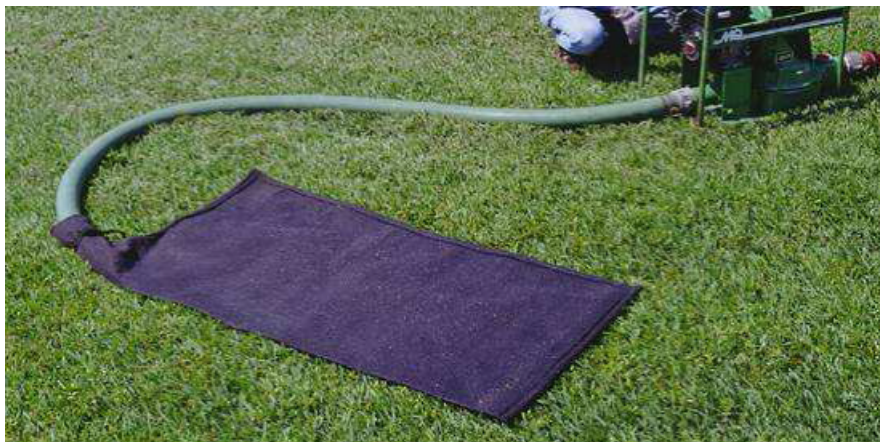
Photograph CS-2 – Example of Dewatering Bag
